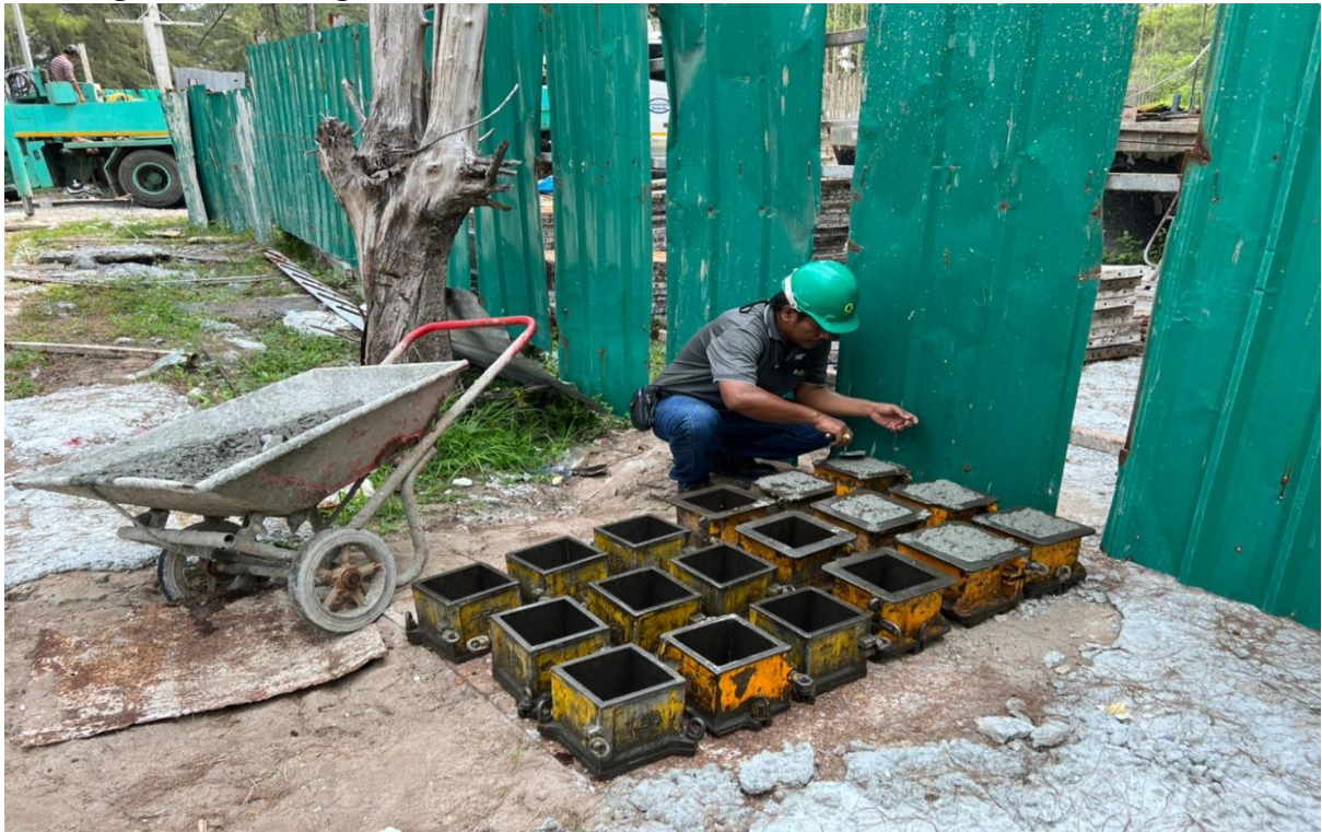
Concrete Compression test moulds being prepared from batches of the salt concrete
