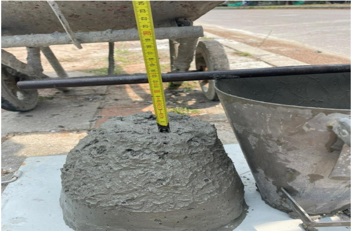
Slump testing random batches of the Concrete during pour
