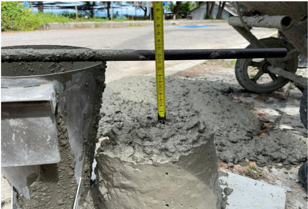
Sampling concrete from the deliveries (Slump test)
