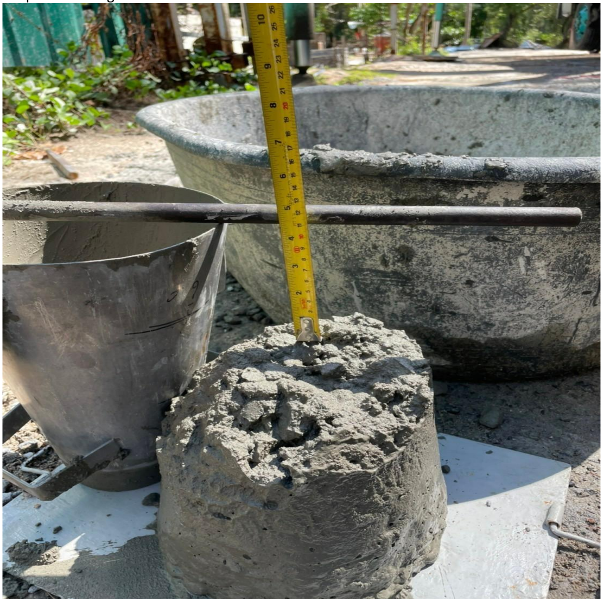
Slump test random concrete batches from readymix when pouring slabs
