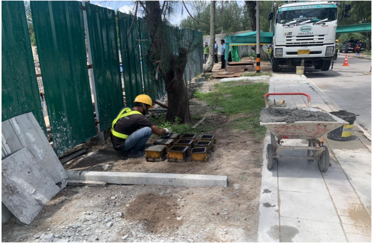
Slump testing and compression test moulds, each batch is tested for slump and randomly for compression test
